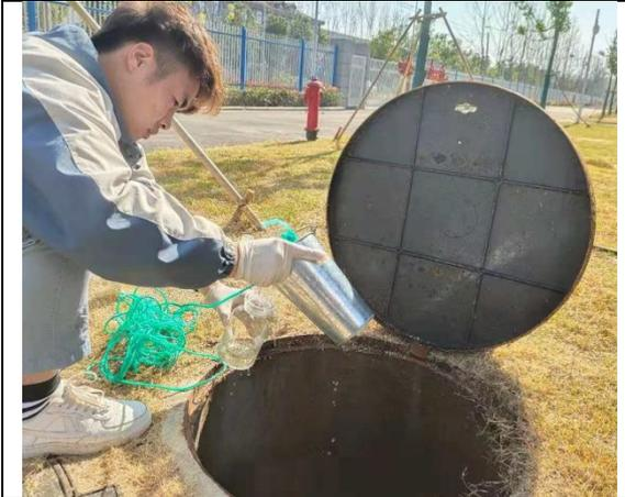
A person in a blue and white jacket is using a silver container to collect a water sample from a large black circular opening in the ground. A green net is visible nearby.                      | <p>/</p>                                                                                                                                                                                                                                                                               |
