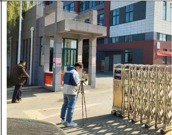
A person in a blue and white jacket is using a tripod-mounted noise meter to monitor noise levels at a gate. A building is visible in the background.                                              |
